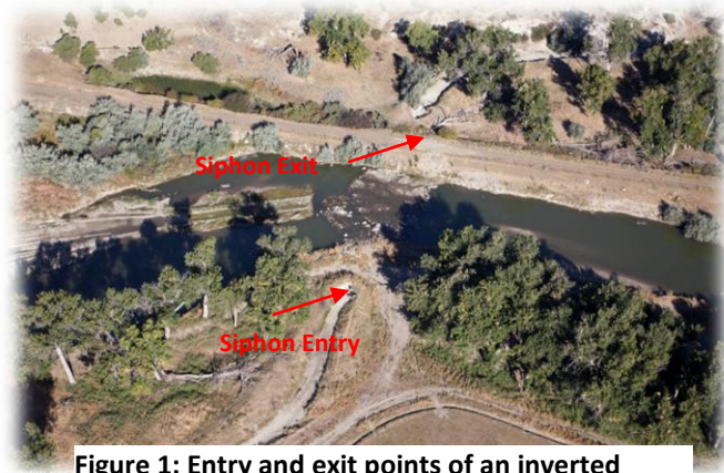
Figure 1: Entry and exit points of an inverted siphon on the Musselshell River.
