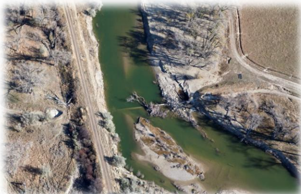
Figure 2: 2011 flood scoured the river bed, exposing the irrigation inverted siphon on the Musselshell River.
