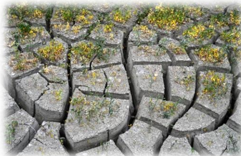
Figure 4. Silt and clay deposits crack deeply after initial drying but cracks won't persist. Photo Credit: Tom Pick
