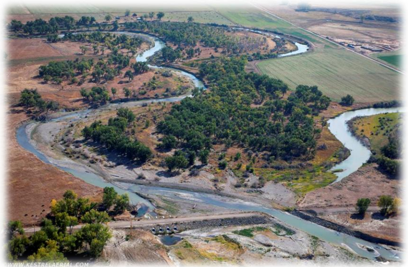
Figure 5. View downstream of Harvey Road Bridge site showing newly constructed high flow culverts to left of channel.
