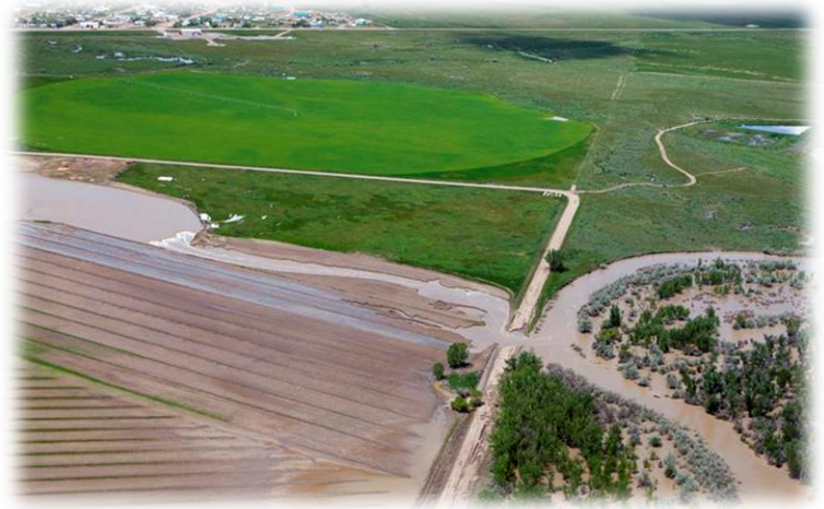
Figure 3. Breached road prism and upstream erosion.
